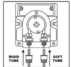
Connect the soft tube to the pump (impulsion – arrow downwards). The injection fitting will be placed at the end of this tube only to inject into a piping. (This fitting has a thread that links it to the piping.)
