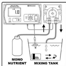
Connect the pump to the MC311 EC controller (on the black and white outlet). The pump will discharge 0,08 cL every 2 seconds when active.
