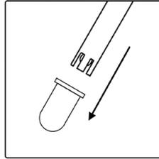
Immerse the tip (2.5 cm) of the EC probe into the sample. (for example it can float with the help of a piece of polystyrol).
