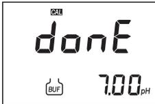
This prompt appears for a few seconds before returning to the main screen, when the pH calibration is done.
