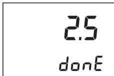
The titration result, expressed as concentration of tartaric acid in g/L, is displayed at the end of the titration process. Press the **START STOP** button to return to the main screen.
