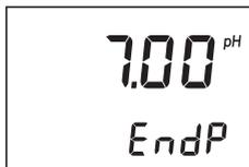
This screen appears when the meter is in main screen and the **pH** button is pressed. Press the **CAL** button in order to change the end-point. Each time the **pH** button is pressed the end point value is changed and the meter returns to the main screen.
