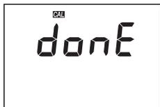
This screen appears for a few seconds before returning to the main screen, when pump calibration is done.
