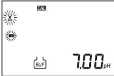
This screen appears when the pH calibration is started by pressing the pH button. Pressing again **pH** or the **CAL** button, the pH calibration is aborted and the instrument returns to the main screen.
